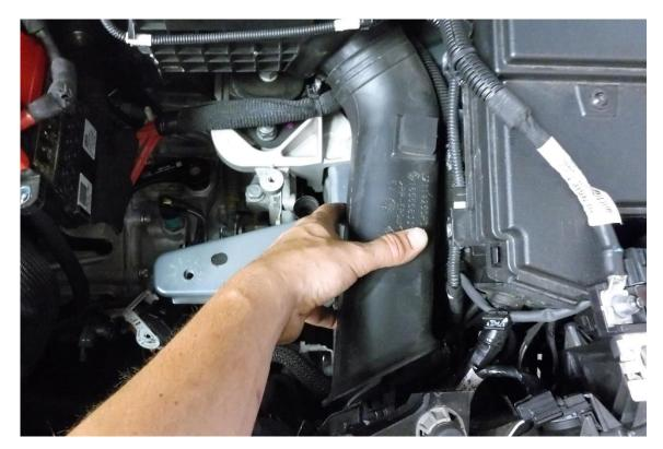
**10**. Unplug the MAF and disconnect the MAF wiring loom from the airbox.
