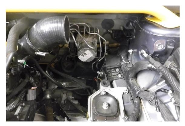
14. Using a T20 Torx drive remove the X2 fasteners attaching the MAF to the OE airbox. Now remove the MAF and reinstall it to the Forge Motorsport MAF boss using the supplied M4 fasteners.
