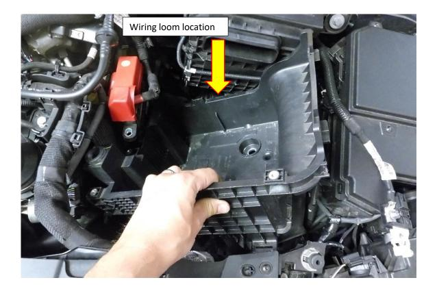
9. Remove the air duct to the airbox, this will simply pull out of the engine bay.
