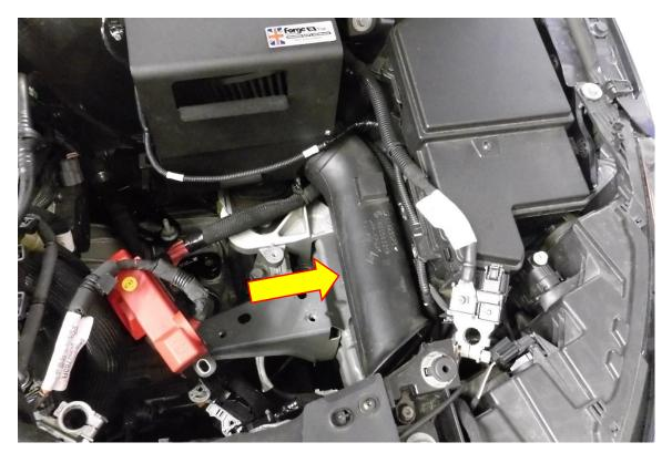
22. Re fit battery tray, when installing make sure the tab on the airbox is sitting on the edge of the battery tray.
