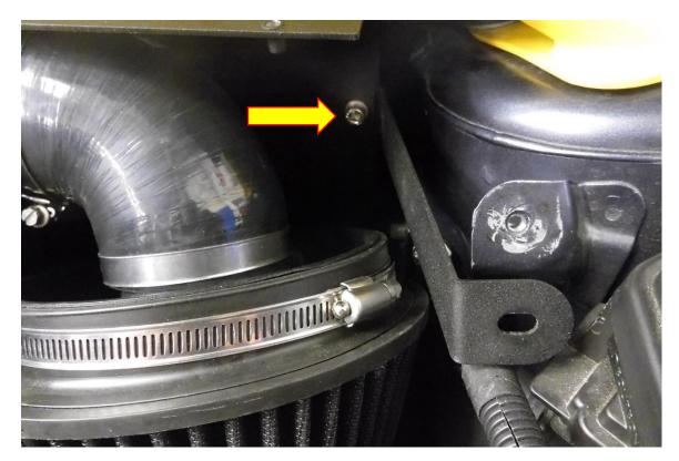
18. Place the airbox complete with air filter and MAF boss into position by locating bottom mounting peg to the rubber mounting point of the original airbox. Fit the MAF to the turbo inlet hose and using the original M6 fastener attach the mounting bracket of the airbox to the vehicle.
