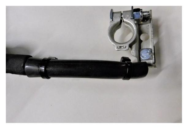
**26**. Fit the POSITIVE battery terminal as shown in the picture below.
