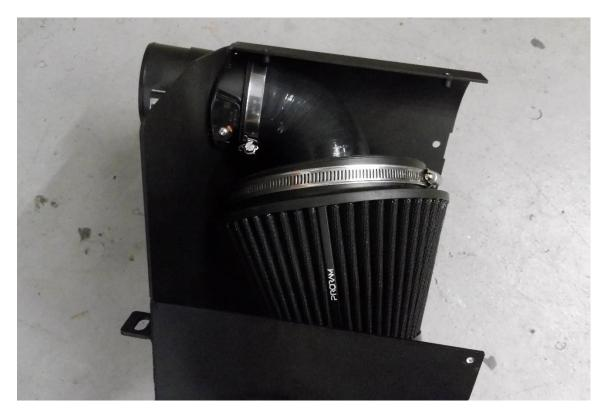
17. Using a 5mm Allen key attach the mounting bracket to the airbox using the supplied M6 x12 fastener and washer.
